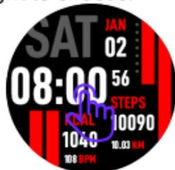
f. Power ON/OFF: Long press power button for 3s to power on; From home page, long press power button 3s, and tap ✓ to power off.
